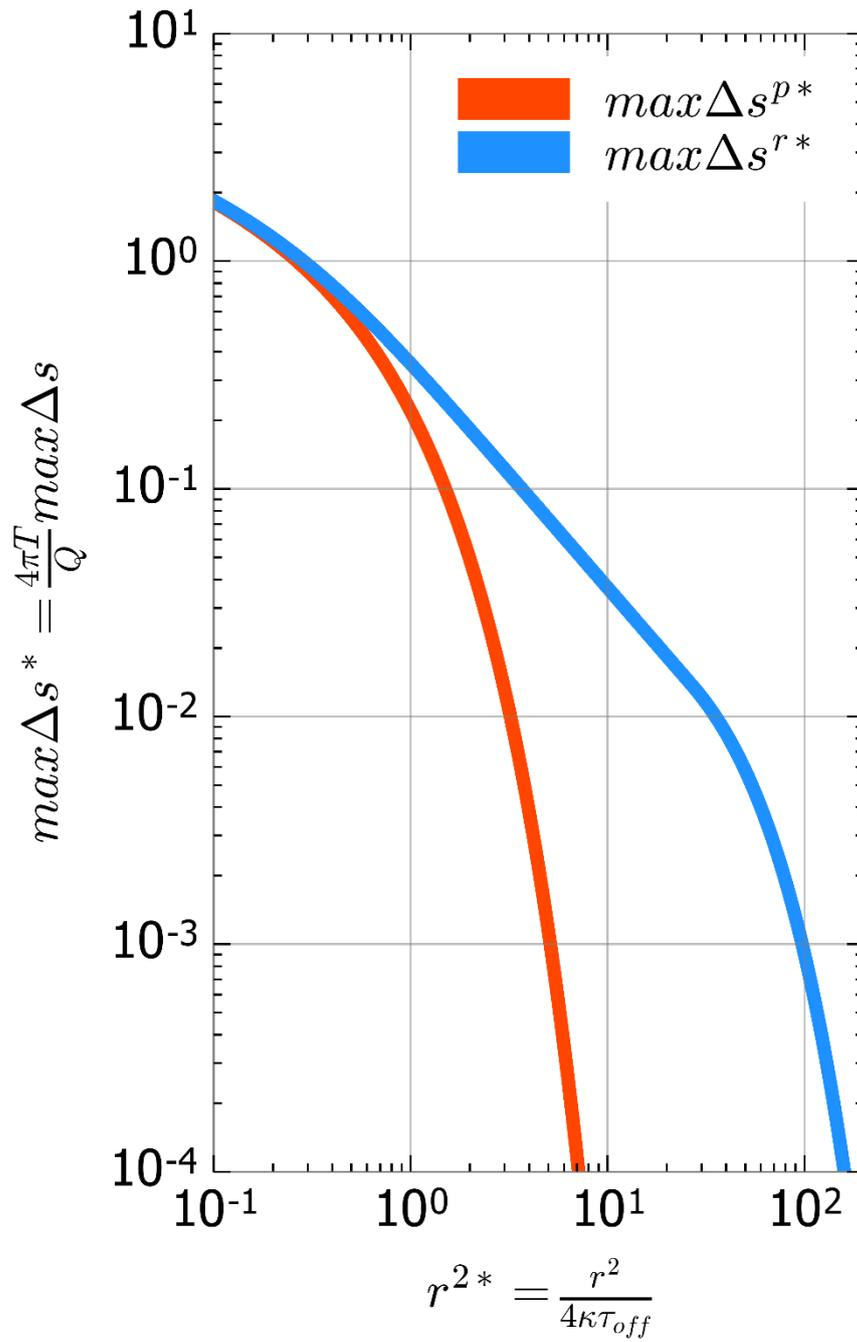
**Figure 3.** Generalised graph of maximum difference in drawdown between the one barrier case and the no barrier case during pumping (in *red*) and recovery (in *blue*), where  $r = R = L$ , as a function of non-dimensional distance ( $r^{2*}$ ).
