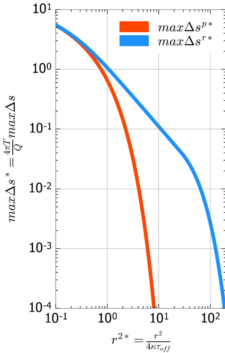
**Figure 7.** Generalised graph of maximum difference in drawdown between the two orthogonal barriers case and the no barrier case during pumping (in *red*) and recovery (in *blue*), where  $r = R = L$ , as a function of non-dimensional distance ( $r^{2*}$ ).
