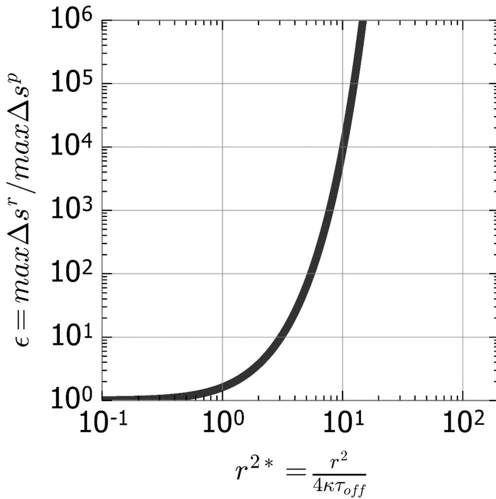
**Figure 4.** Generalised graph of the ratio of the maximum difference in drawdown between the barrier and no barrier case during pumping compared to recovery ( $\epsilon$ ), where  $r = R = L$ , as a function of  $r^{2*}$ .
